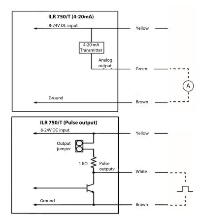
Figure 20: ILR 750, 750T wiring
