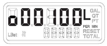
Figure 12: Pulse rate out screen
