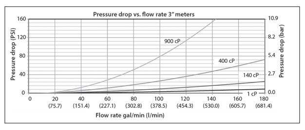
Figure 2: Pressure drop vs. flow
