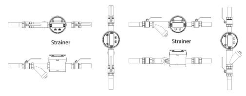
Figure 1: Meter installation
