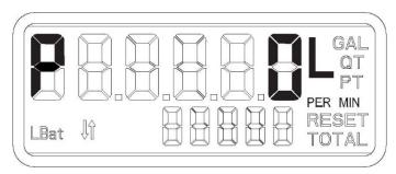
Figure 11: Output pulse length screen
