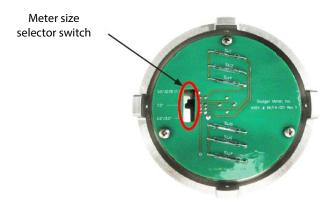
Figure 18: ILR 741 transmitter switch positions
