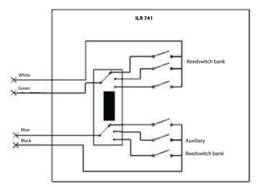
Figure 19: ILR 741 wiring
