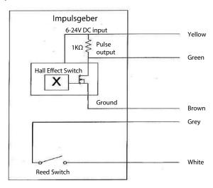
Figure 21: ¼" and ¼" low flow wiring
