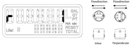
Figure 7: Register orientation
