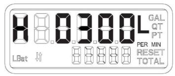
Figure 10: Analog maximum flow rate screen
