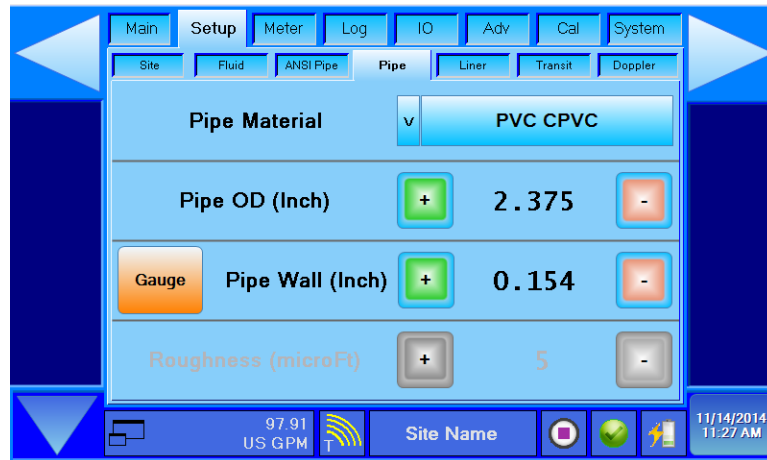
Figure 55: Pipe page allowing manual entry
