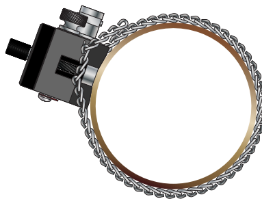
Figure 30: DTTSU transducers mounted
