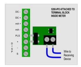
The pulse output built into CDI flowmeters is an opencollector transistor output that functions as a switch to the meter's ground. It does not provide electrical isolation between the meter and the receiving device. The IPO provides this isolation.
