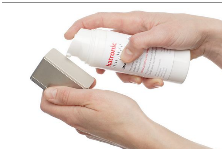
Picture 8: Application of acoustic coupling gel
