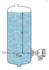
P<sub>hydr</sub> [bar] = hydrostatic pressure
