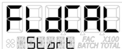
If “Start” is in focus when advancing to the next menu, the software will automatically advance to the calibration menu for the calibration method the user previously selected.
