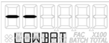
Note: If the battery life is sufficiently low, "LOWBAT" will be displayed in the message area on the bottom row of characters. This low battery message will be displayed automatically without running a diagnostic battery check.
