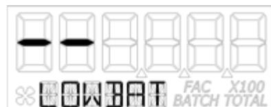
**NOTE:** If the battery life is sufficiently low, "LOWBAT" will be displayed in the information row. This low battery message will be displayed automatically without running a diagnostic battery check.
