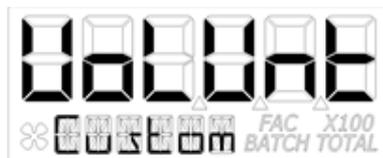
The software also allows the user to create their own “Custom” volume unit (see Figure 19). Advancing to the next menu with the “Custom” volume unit in focus will shunt the user to a new menu (see below) that will allow the user to create a new label, or reuse one already stored in computer memory.
