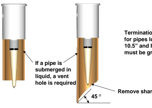
**Termination** is required for pipes longer than 10.5" and ID of pipes must be greater than 6"
