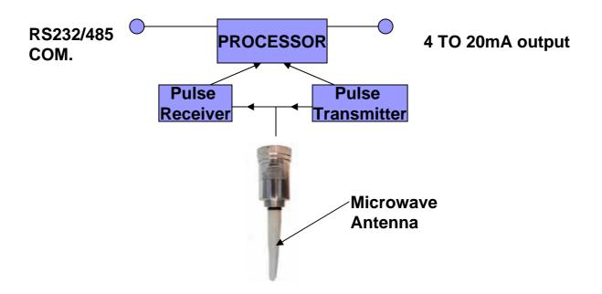
Microwave rod antenna is stimulated by an electromagnetic pulse transmitter and sends very short pulses to a target. They reflect from a target and then they are received by the same antenna. The electrical signal from the antenna is amplified and processed. Distance to an object is calculated and converted to 4mA to 20mA and also optionally, level information is sent to a PC via RS232 or RS485 for diagnostic data logging and programmable set-up.
